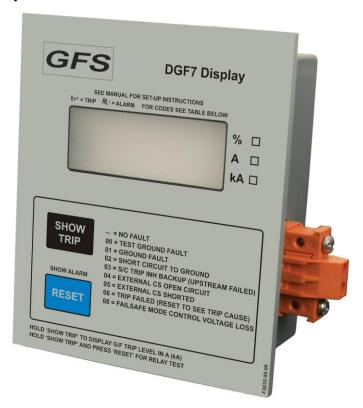
The door mounted DGF7 Display is connected to the DGF7-3 by up to 5 m of cable (shielded cable if longer than one meter). It provides the following remote indications and functions:
